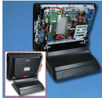
Tool-Free Access Optimizes Serviceability
