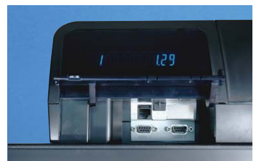
Up to Three RS-232C Ports Hidden Behind a Convenient, Easy to Access Door
