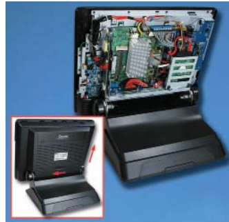
Tool-Free Access Optimizes Serviceability
